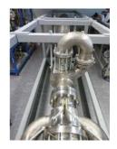
The TA-engine is located at the left side and generates acoustic power from a stream of waste heat stream at a temperature of 140 °C. The acoustic power flows through the resonator to the TA-heat pump, located on top of the resonator. Waste heat of 140 °C is upgraded to 180 °C in this component. The total system can be generally applied into the existing utility system at an industrial site.
